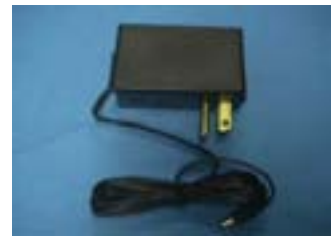
G – Battery Charger
