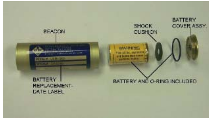
FIGURE 3. BEACON EXPLODED VIEW SHOWING RELATIVE LOCATION OF BATTERY AND RELATED PARTS
