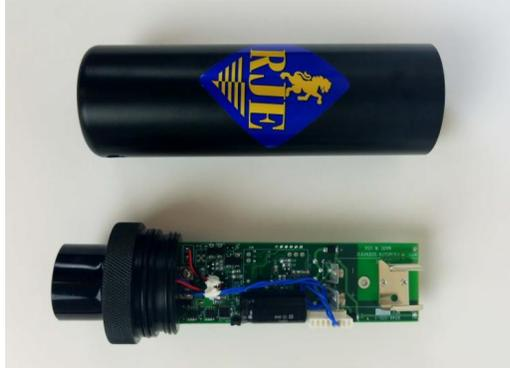
Figure 4-1 ULB-364 Disassembled
