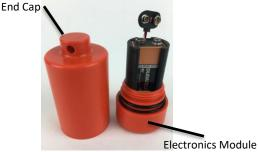
The ULB-350 series beacon can be mounted using the mounting hole at the center of the end cap or strapped to the item to be marked. Always try to mount the ULB-350 vertically in the water column, with the end cap pointed down and the electronics module facing up. Insure that the electronics module is free of obstruction so that it has a clear path to send the acoustic signal through the water.
