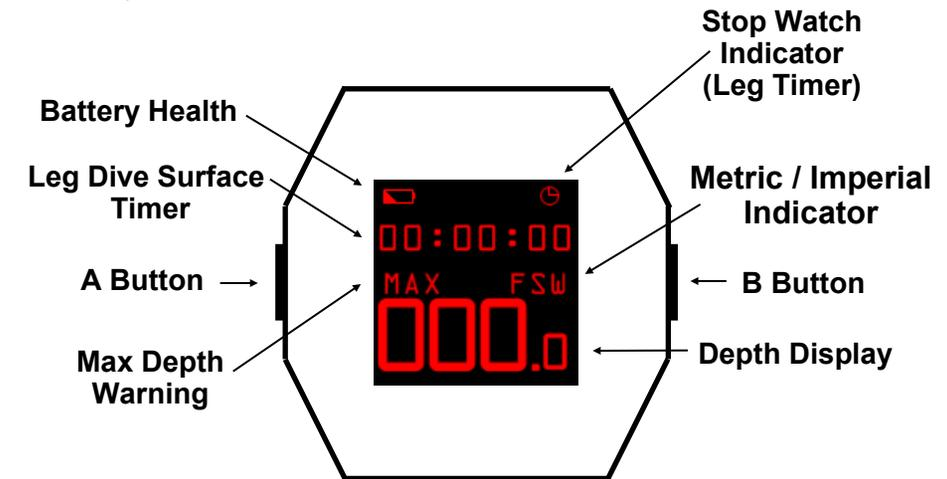
Depth readings are provided to the diver through a large Red OLED display on the bottom of the screen. Both dive and leg times are displayed at the top of the screen. The DG100 buttons supply access to these functions. All functions of the DG100 are controlled through buttons on each side of the display. Buttons are operated in two modes: Short Press or Long Press. Short Press is defined as less than 1 second. Long Press is defined as lasting 2 seconds or more.
